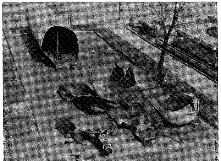
Figure 2. Partly "reconstructed" tank car from the Crete, Neb. accident.
